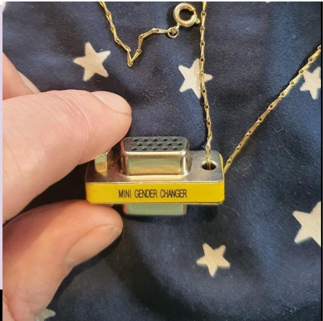
Female Gender Changer (two sides with pin holes -female) talisman gifted to the graduate of the GCA. This socket typically connects to a Male Gender Changer (two sides with pins -male). Image: NM-F
